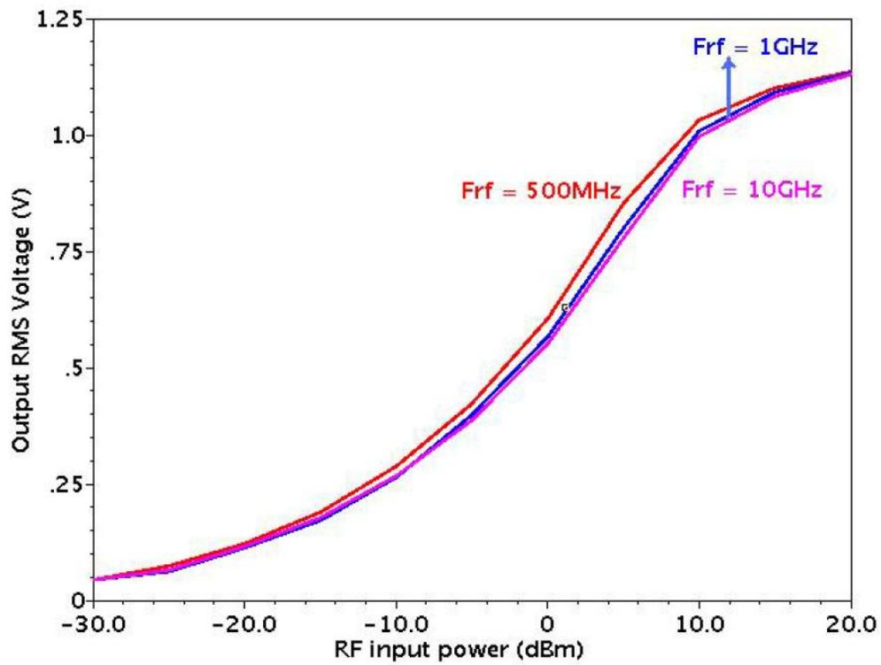
Fig. 6. Characterization of the envelope detector.
