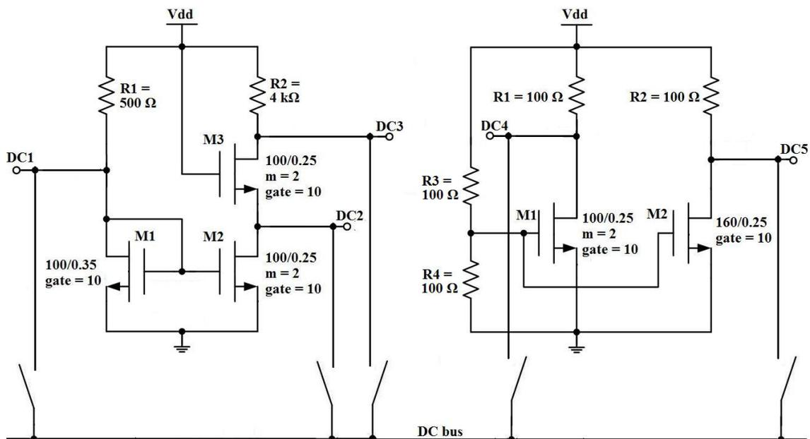
Fig. 1. Fictif/Dummy circuits: (a) polarization circuit with a current mirror and (b) Gain stages with different geometries.
