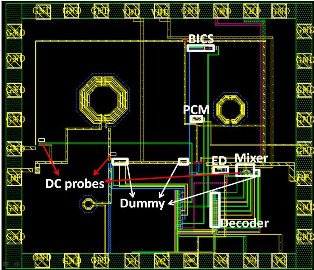
Fig. 5. Layout of the Chip
