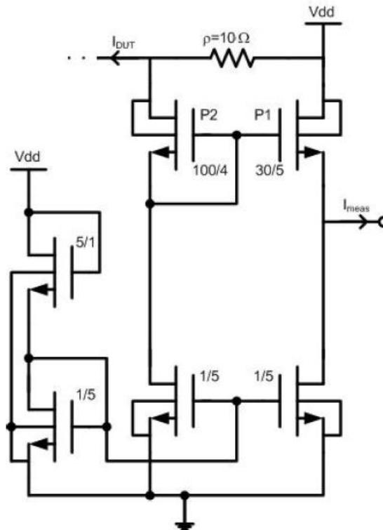
Fig. 3. CMOS Current Sensor
