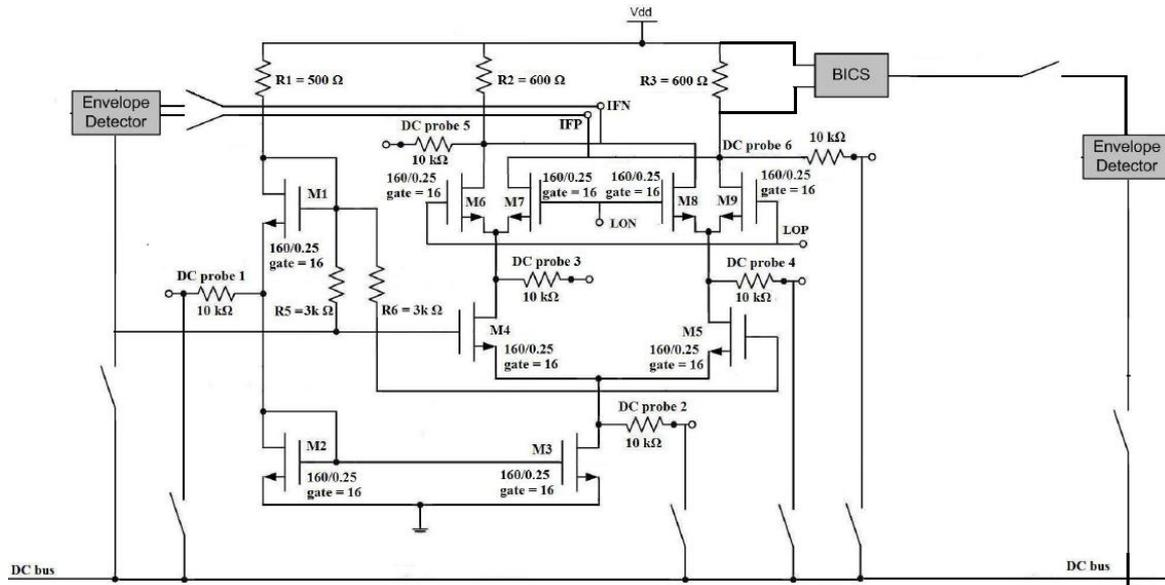
Fig. 4. The electrical scheme of the RF Mixer with on-board monitors.
