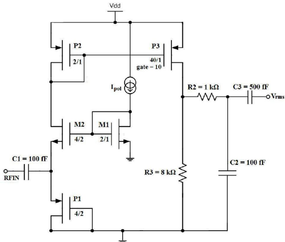
Fig. 2. CMOS Envelope Detector
